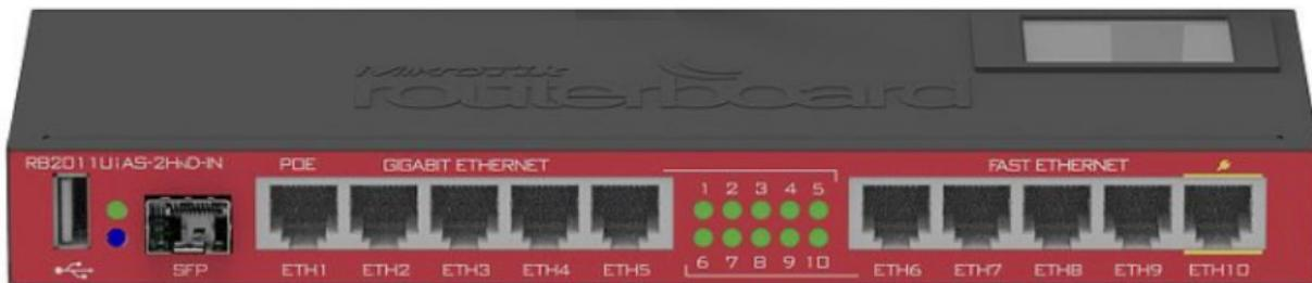
RouterBOARD 2011UiAS-2HnD has most features and interfaces from all our Wireless routers. It's powered by the new Atheros 600MHz 74K MIPS network processor, has 128MB RAM, five Gigabit LAN ports, five Fast Ethernet LAN ports and SFP cage (SFP module not included!). Also, it features powerful (up to 1W!) dual chain 2.4Ghz 802.11bgn wireless, RJ45 serial port, full-size USB port, and RouterOS L5 license.
