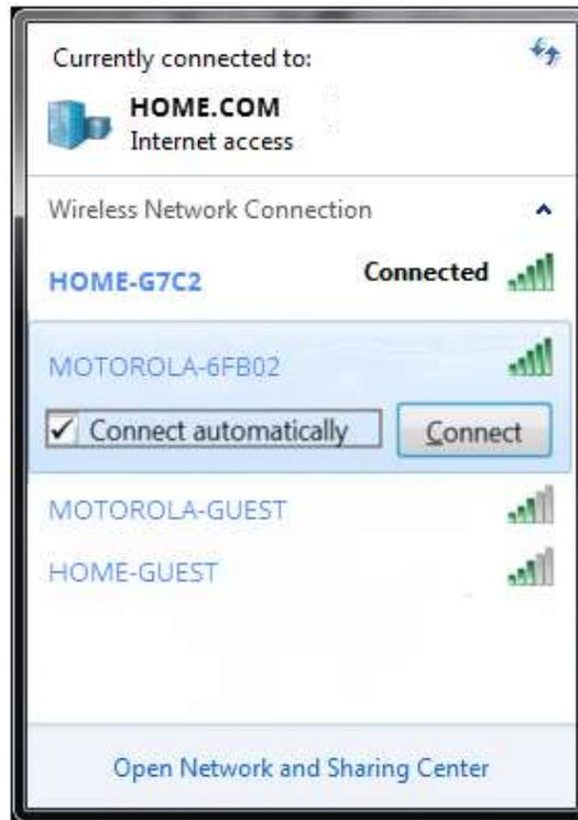
Figure 19: Sample Wireless Network Connect Window
